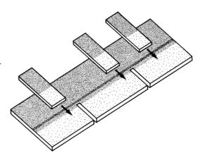
Whereas Shangle consists of a full-size, onepiece base shingle onto which tabs or pads are applied, a two-piece laminate uses a full-size shingle with tab-size teeth cut out of it. Adhered to the back of this top shingle is a half shingle that runs behind the cut-outs. The result is a multi-layered shingle that provides a rugged, textured look on the roof.
